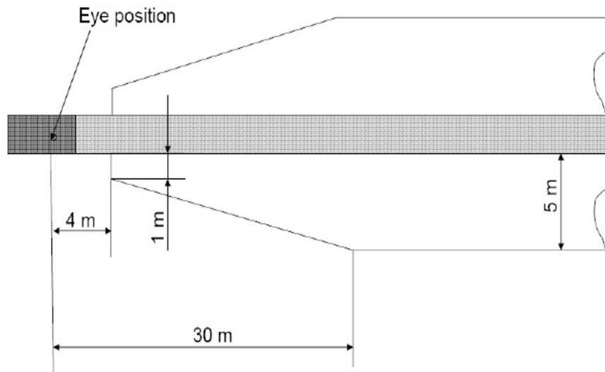
Figure 1-Field of vision laterally behind the vehicle (ISO 5721-2)
