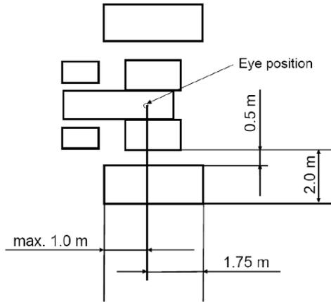
Figure 2 Field of vision beside the vehicle in 1m height above the ground
