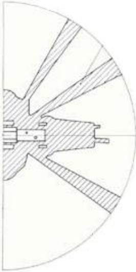
ISO (International Standards Organization) Standard 5721 (1989) requires in summary, a light source being used to replace the operator's eyes. From the position of the eye location of the operator in the driver's seat the areas not shown by the light are diagrammed, and this is illustrated by the shaded area in Figure 1 showing the lack of visibility around the area of the tractor.
