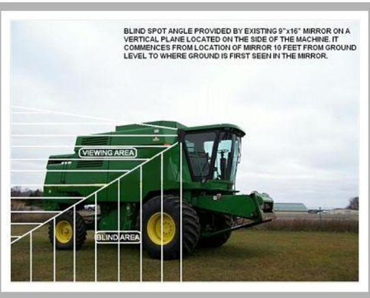
The photos also illustrate the problem of proper location of the mirrors on the vehicle. The mirrors should be located if possible to the front of the operator so they can be checked by a glance while maintaining the eyes to the front area of the vehicle.
