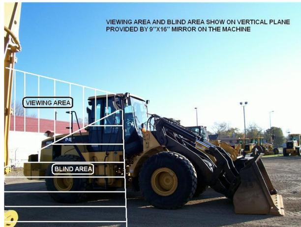
**The mirror does not show the ground at the immediate rear of the machine and leaves a vertical blind spot along the side of the unit at the rear so there is non-compliance with 14401 and 5006.**
