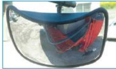
**The distortion factor would be so great that the driver would be unable to identify what is being shown.**
