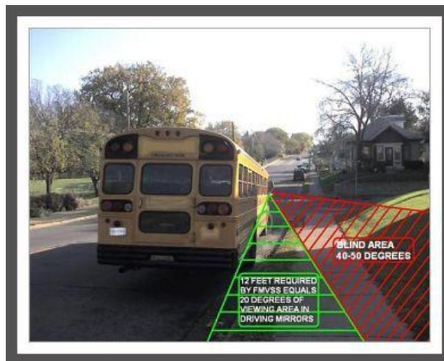
It is submitted that this horizontal plane blind spot requires the operator to turn and look into this area to safely make a lane change or turning maneuver and while doing so is required to take the eyes off the road ahead and possible upcoming obstacles. This blind spot also cannot be corrected except by bending the glass further making the distortion factor a greater problem.
