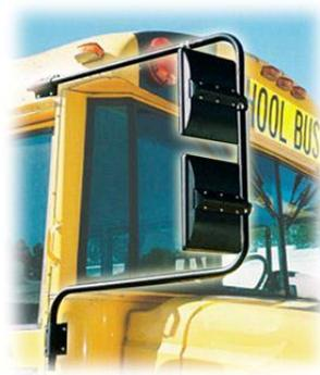
More recent innovations have included a case type mirror where both the flat glass and the convex glass are contained in the same case. (Figure 4 illustrates such a mirror).
