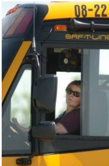
During this procedure the operator is not viewing the area upcoming and the potential for an accident is greatly enhanced. Further placing the mirrors in front of the driver can reduce the problem of mirror clipping which is becoming more of a problem as operators stick the mirrors out further on the side of the bus to increase the field of view for the operator.
