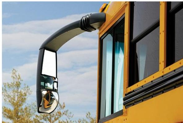
If we assume, which is what we found in actual studies, that the operator of the school bus is being provided with exterior mirrors on the passenger side of the bus that provide a view of the area 12 feet out from the center of the rear axle of the bus on the passenger side, we can examine the quality of that view as an aid to successfully operate the bus during the normal school day.
