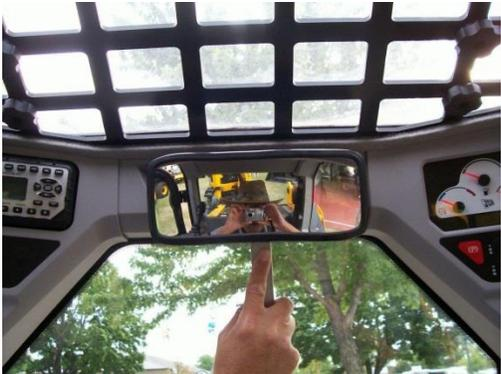
Note the size of the vehicle behind the skid-steer in both photos, with the standard convex mirror the unit immediately behind the subject vehicle appears to show the unit much farther away from the subject vehicle than it really is.
