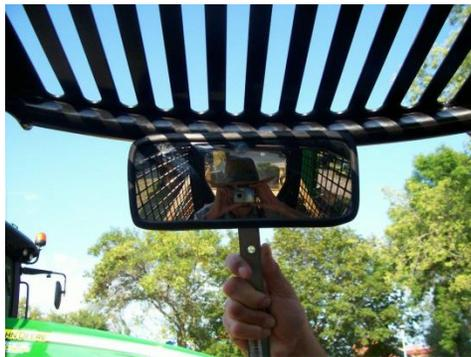
On a less severe Falling Object Protective Structure (FOPS) and no side curtains the full benefit to be achieved with the use of the M-C Mirror is illustrated by the below photo;
