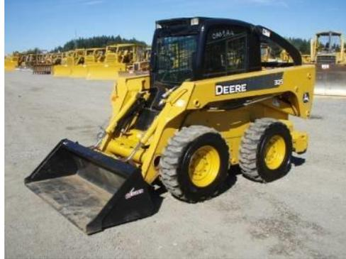
Skid-Steer machines are designed to make quick movements in all directions, going backwards and forwards and turning every few seconds. Due to their design, skid-steer machine loaders have compromised vision to the side and to the rear with large blind spots at the rear. The blind spots can be illustrated by the following diagram:
