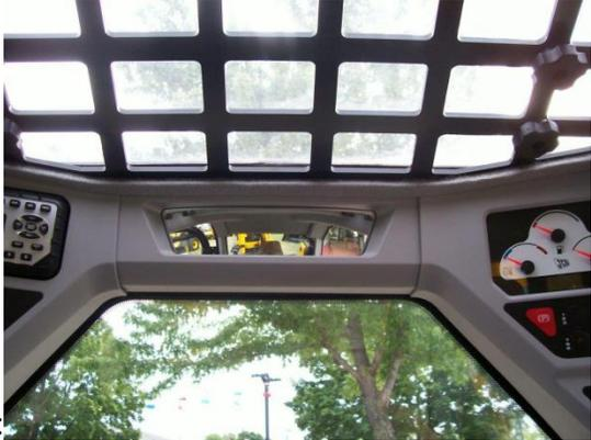
Sitting in the driver's seat illustrates that this solution provides minimum help to the operator primarily because the mirror technology being used is a wide angle standard convex mirror, which produces images smaller than normal so the operator cannot make them out clearly. Also note that the size of the mirror itself is too small to offer the operator the best view possible.
